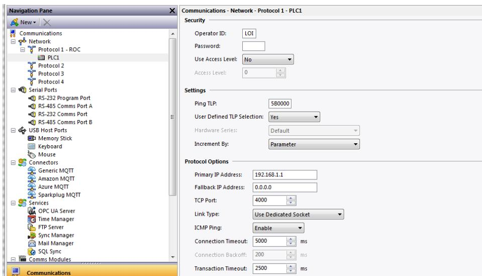
Note - Only configure the Fallback IP Address (C3.1+ only) if there is a secondary ROC IP address for redundancy communications.
