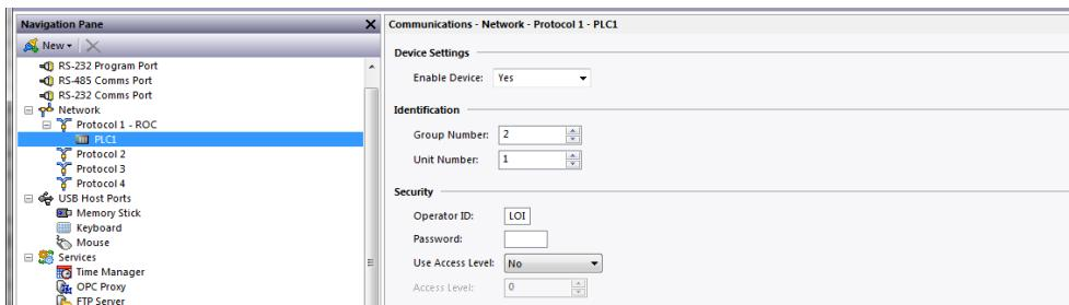
Please specify the Operator ID and Password that the Red Lion device should use when communicating with the ROC device. Also, indicate the Access Level if any.
