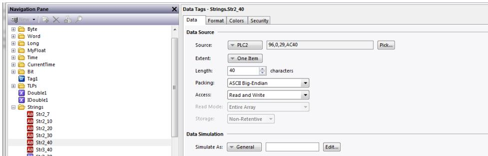
If the string tag is not initially set to the proper length, the communication blocks may need to be rebuilt. This can be accomplished by running the Rebuild Comms Blocks utility available in Crimson’s File->Utility menu.
