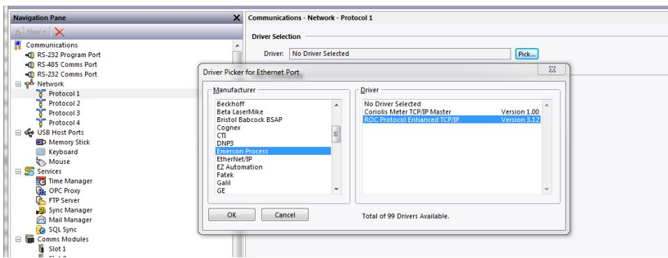
Find the Emerson Process ROC Protocol Enhanced TCP/IP communications driver as shown above and click OK. Next select the PLC device and configure the IP address and the TCP Port such that it matches the configuration in the ROCLINK 800 software.
