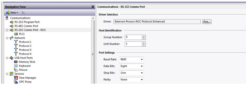
Modify the Baud Rate, Data Bits, Stop Bits and Parity settings such that it mirrors the port settings in the ROCLINK 800 software.
