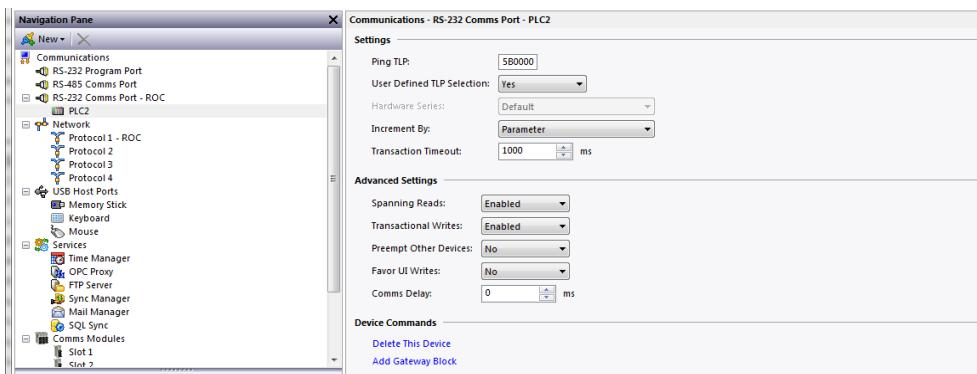
The first field provides the ability to select a Ping TLP. This TLP should contain only 1 byte of data (UINT8) and should always be available in the target device. Enter this value in the format of TTLLPP where TT is the Point Type, LL is the Logical Number and PP is the parameter in hexadecimal form.
