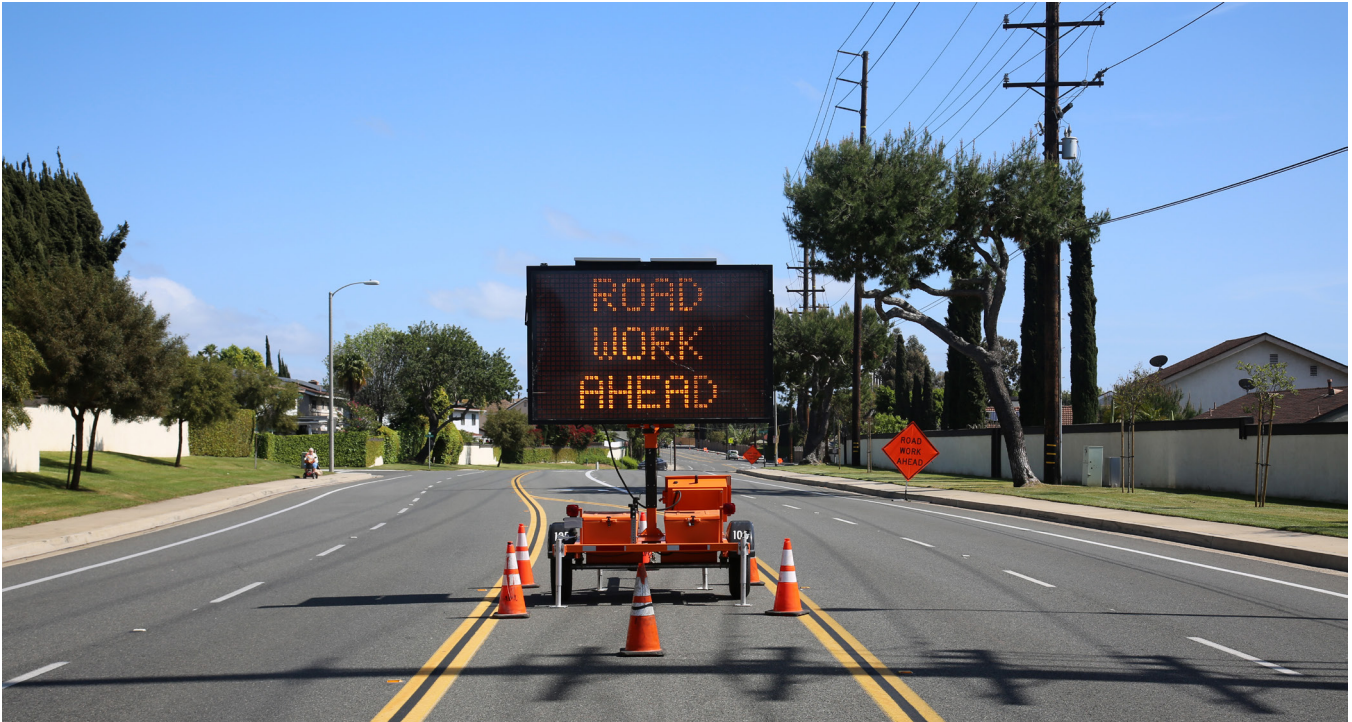
Figure 9. Battery powered traffic sign with an internet connection
