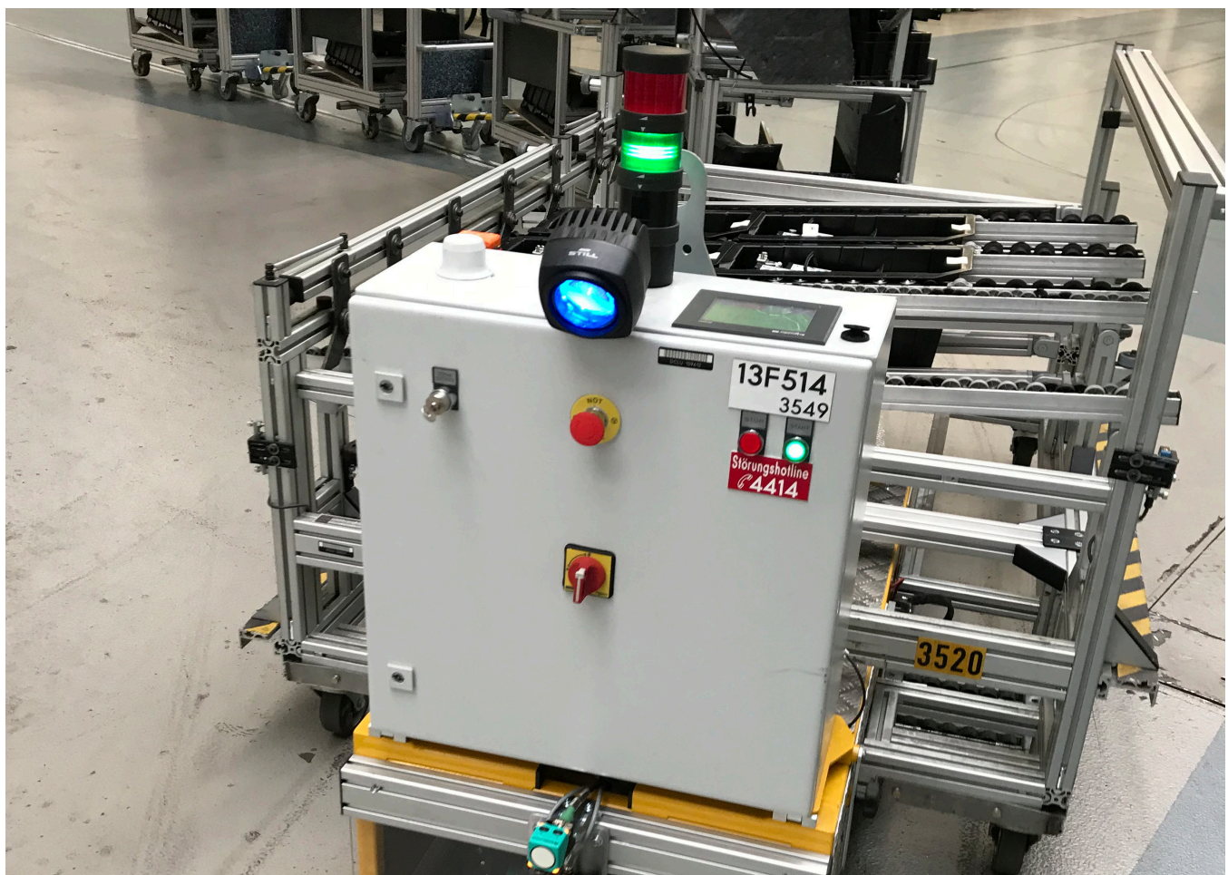
Figure 8. The Anybus Wireless Bolt is attached to an AGV and uses Bluetooth technology to safely move around the factory
