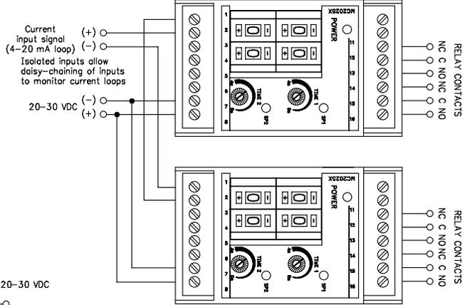
Typical current loop installation:
