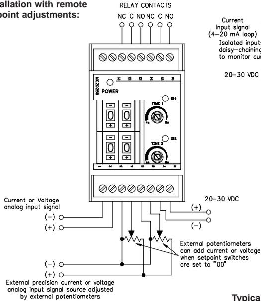
Typical dual module installation:
