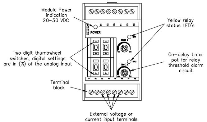
The same example can be applied to 0 to 20 mA analog input signals. Introducing an external mA signal now increases the threshold trip point.
