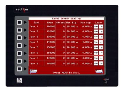
Each level input must be scaled to accurately measure the contents of the tank. The Span is the value that will be displayed when the Maximum Signal is reached, and the Offset is the value that will be displayed when the Minimum Signal is reached.
