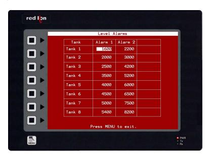
The alarms menu shows the values, in lbs., at which the alarms will energize. To change a value, simply press it, and a numeric keypad will pop up. Type in the new alarm value, and press Enter.
