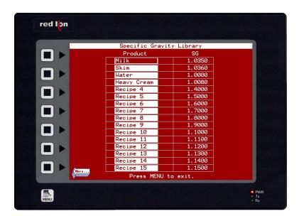
The Specific Gravity Library provides the means to store up to 16 different liquids, as well as their specific gravity. This allows the operator to assign various liquids to different tanks by name, instead of by specific gravity. (See Selecting a Product.)
