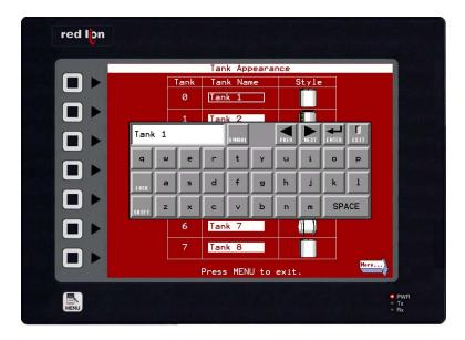
The first page of the Initial Setup menu allows you to enter a meaningful name for each of the tanks, as well as choose a tank graphic for each. To change the tank name, simply double-tap the desired field, and an alphanumeric keypad will appear. To change a tank's graphic representation, touch the tank next to the name.
