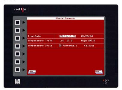
The Miscellaneous page allows the adjustment of several parameters that are loosely related. The time and date may be adjusted, which is important for the historical trending and data logging features.
