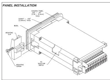
The unit meets NEMA 4/IP65 requirements for indoor use, when properly installed. The units are intended to be mounted into an enclosed panel with a gasket to provide a water-tight seal. Two mounting clips and screws are provided for easy installation. Consideration should be given to the thickness of the panel. A panel which is too thin may distort and not provide a water-tight seal. Recommended minimum panel thickness is 1/8".)
