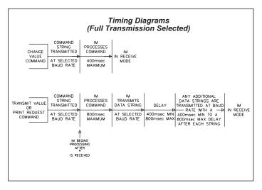
Note: If Full Transmission is selected and the front panel is being accessed at the time of transmission, the IM may take as long as 2 seconds to respond.
