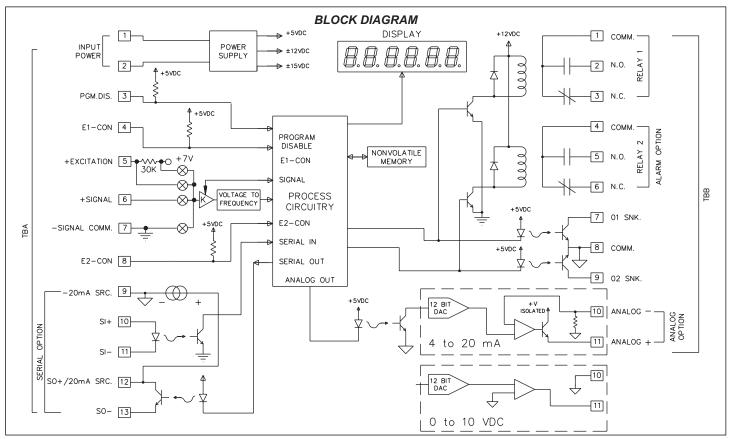
Note: Analog "-" and Alarm common are separate and isolated from the signal common. The commons should NOT be tied together.
