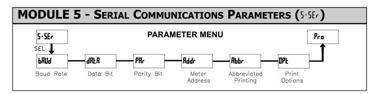
Module 5 is the programming module for the Serial Communications Parameters. These parameters are used to match the serial settings of the CUB5 with those of the host computer or other serial device. The Serial Setup Parameters are only accessible when an optional RS232 or RS485 serial communications module is installed in the meter.
