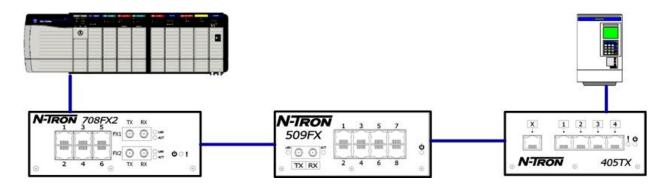
In the above network there are three switches: 700, 500, & 400 all in series. There is a PLC connected at one end and a drive connected to the other end. In order for the PLC to communicate with the drive, data must pass through all three switches. Therefore each of the switches availability must be included in the network's availability.
