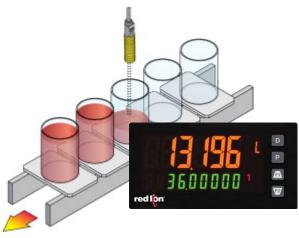
Proper material level is essential to a production line to insure every product is properly packaged. The PAX2A can accept the input from an ultrasonic sensor and stop the filling process when the liquid reaches the proper height. Using the PAX2A as the controlling device, the setpoint can provide the stop once that level is reached. The top line can indicate the actual level during the filling process, while the bottom line displays the goal or setpoint.
