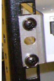
3. Install the switch into your rack using standard rack hardware not included with the switch. Alternatively, you can skip the rack installation if you would like to configure the switch beforehand.
