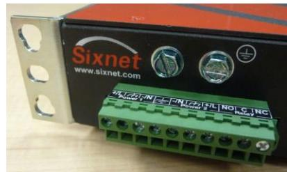
**IMPORTANT NOTE:** Make sure to turn off your power before making any connections to the switch. Make sure you are applying the correct power to the correct screws. Follow all local, national or regulatory rules that apply.
